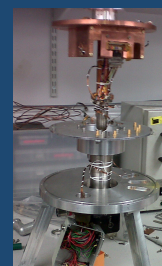
Figure Above: Southern C-BASS receiver schematic. Figure Right: Southern receiver cold stages, bottom plate will be at 40 K whilst the top plate will be at 10 K.
