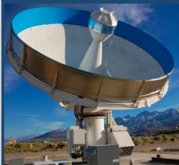
Figure Left: Northern C-BASS Figure Below: Sidelobe measurements for Northern C-BASS without any baffles at all (black), with only the secondary /inner baffle (grey) and with both inner cone and outer rim baffles (dotted black). Holler et al (2012), arXiv:1111.2702.
