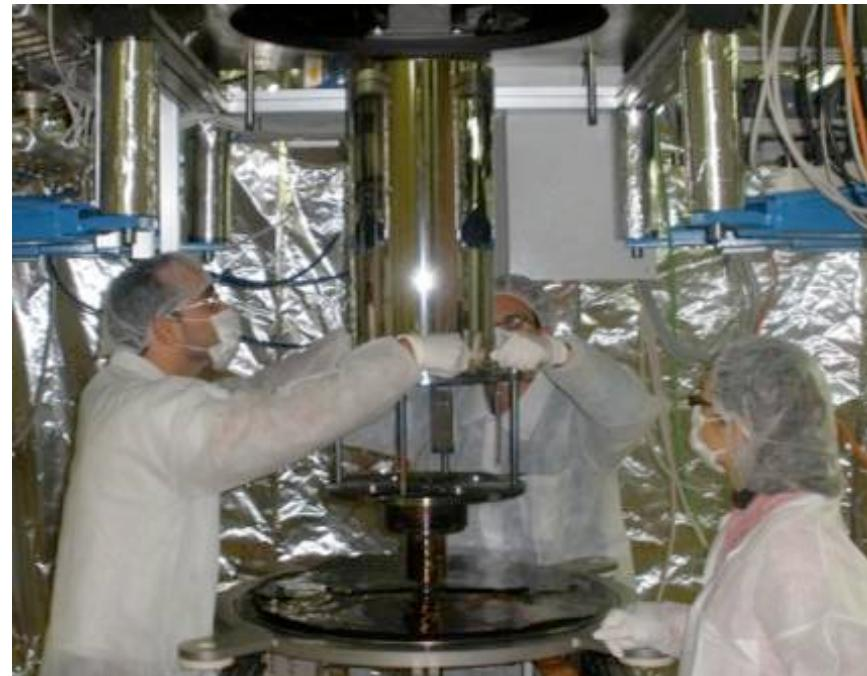
The multilayer is deposited on the electroformed shell on top of the gold surface
