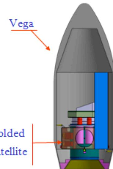
Figure 28: The folded satellite inside the VEGA fairing
